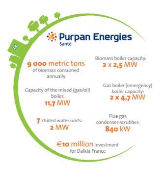
The boiler plant will have two 2.5 MW wood-fired boilers that will provide 90% of the site's heat requirements. A condensation heat recovery system, a very efficient solution in energy terms, will recover the energy from the condensation of the plant's flue gas. This new boiler will consume 9,000 metric tons of wood fuel a year sourced from the local forestry industry.
